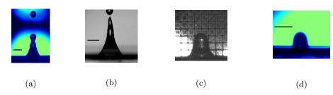
Figure 11: Images of jets for different conditions giving an idea of the effect of Bond number and viscosity. (a) Bubble of R=2.15 mm in water, Bo=0.629,  $Oh=2.55 \times 10^{-3}$ ; (b) R=2 mm in GW48 (30°C), Bo=0.646,  $Oh=10 \times 10^{-3}$ ; (c) R=4.08 mm in water, Bo=2.25,  $Oh=1.85 \times 10^{-3}$ ; (d) R=1.46 mm in GW72, Bo=0.39,  $Oh=4.9 \times 10^{-2}$ . The lines in images 11a, 11b and 11d are 1 mm in length. The grid size in image 11c is 1 mm.
