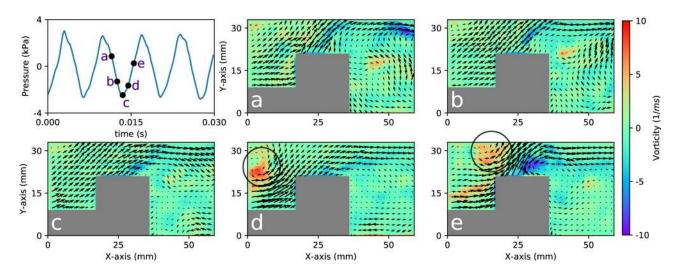
FIG. 4. Instantaneous snapshots of the vorticity field superimposed on the velocity field corresponding to the points (a)-(e) marked on the time series of fluctuating pressure during thermoacoustic instability.
