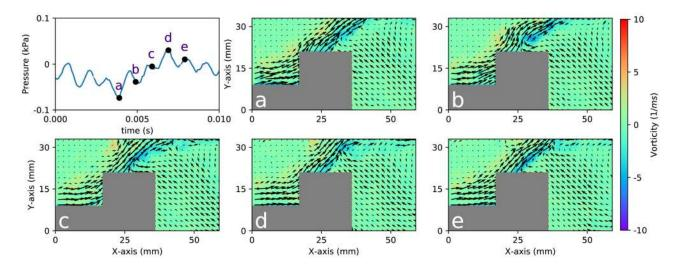
FIG. 2. Instantaneous snapshots of the vorticity field superimposed on the velocity field corresponding to the points (a)–(e) marked on the time series of fluctuating pressure during combustion noise.
