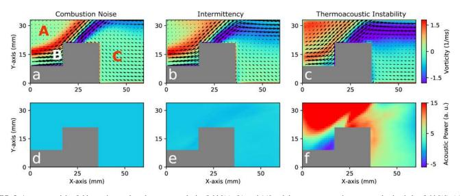
FIG. 5. Average vorticity field superimposed on the average velocity field [(a), (b), and (c)] and the average acoustic power production index field [(d), (e), and (f)] during combustion noise, intermittency, and thermoacoustic instability. During thermoacoustic instability, regions of high average acoustic power production coincide with regions of high average vorticity present in the wake of the dump plane upstream of the bluff body.
