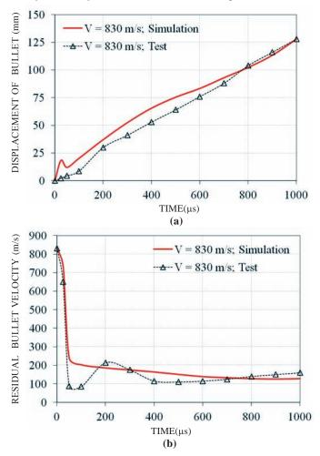
Figure 6. Displacement and residual velocity of AP shot in Case-2 analysis : (a) Displacement and (b) Residual velocity.
