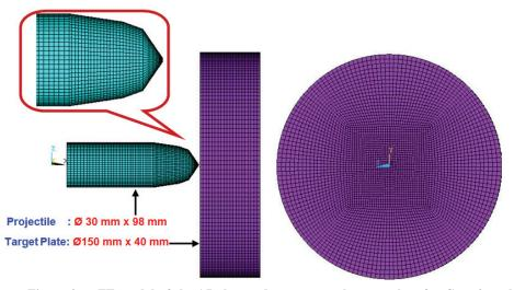
Figure 2. FE model of the AP shot and armour steel target plate for Case-2 analysis.
