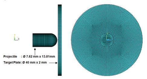
Figure 1. FE model of the bullet and target door plate for Case-1 analysis.
