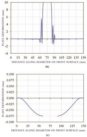
Figure 5. Deformation in target plate in Case-2 analysis for V = 830 m/s at t = 1000 µs. (a) Deformed armour plate in Case-2 analysis and test<sup>13</sup>, (b) Lateral deformation at centre, and (c) Lateral deformation away from centre.
