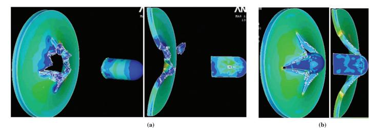
Figure 3. Deformed bullet and target plate at  $t = 50 \ \mu s$ : (a)  $V = 1000 \ m/s$  and (b)  $V = 500 \ m/s$ .
