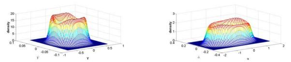
Fig. 10. Joint probability density function of the heave and pitch response respectively for  $U_m = 7.2$  m/s
