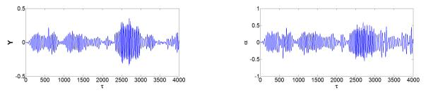
Fig. 7. Time histories of the heave and pitch response respectively for  $U_m = 6$  m/s
