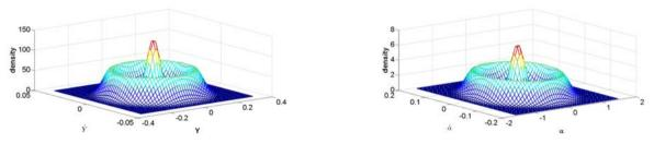
Fig. 8. Joint probability density function of the heave and pitch response respectively for  $U_m = 6$  m/s.
