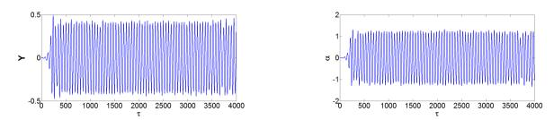
Fig. 9. Time histories of the heave and pitch response respectively for  $U_m = 7.2$  m/s
