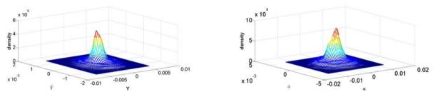
Fig. 4. Joint probability density function of the heave and pitch response respectively for  $U_m = 4$  m/s.
