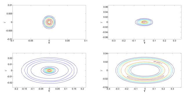
Fig. 11. Contour plot of the heave response and its instantaneous derivative for  $U_m = 4$  m/s,  $U_m = 5.2$  m/s (top row),  $U_m = 6$  m/s and  $U_m = 7.2$  m/s (bottom row) respectively.
