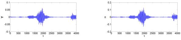
Fig. 5. Time histories of the heave and pitch response respectively for  $U_m = 5.2$  m/s
