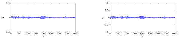
Fig. 3. Time histories of the heave and pitch response respectively for  $U_m = 4$  m/s.
