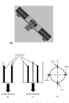
FIG. 2. Experimental schematics. (a) Schematic of the twin-jet setup, (b) microphone arrangement for measuring spanwise instability modes in a single jet, (c) microphone arrangement for measuring spanwise coupling instability modes in twin jets, and (d) microphone arrangement for measuring azimuthal instability modes in an axisymmetric jet (direction of jet flow is out of the plane of the paper).
