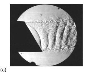
FIG. 1. Schlieren images of shock-containing jets illustrating various spanwise (a) symmetric, (b) antisymmetric, and (c) oblique modes from Raman (Ref. 16).
