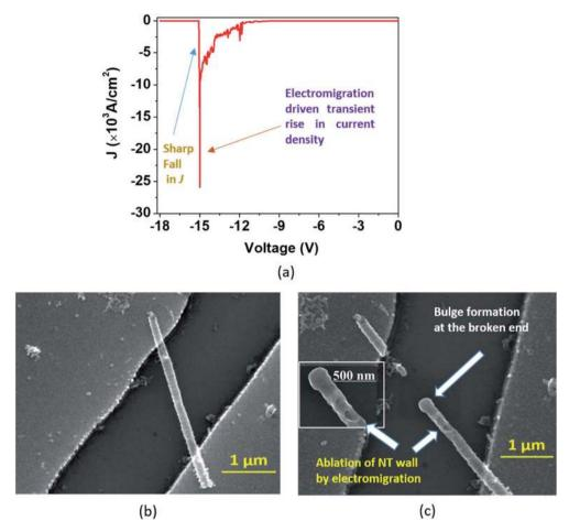
Fig. 7 (a) In the 'Model B' breakdown, the J-V curve displays a sharp transient rise in J before the breakdown point and a sharp fall after the breakdown. SEM images show a single DMTNT (b) before and (c) after the breakdown. Bulge formation occurs at the broken end of the NT due to excessive heat dissipation as shown in (c); magnified image of the broken end in the inset of (c).
