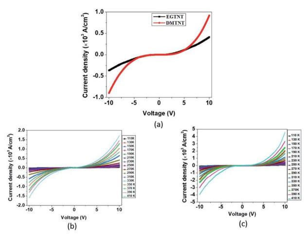
Fig. 2 Current density-voltage (J-V) plots (a) for EGTNT and DMTNT at room temperature, (b) for the individual EGTNT at different temperatures and (c) for the individual DMTNT at different temperatures.
