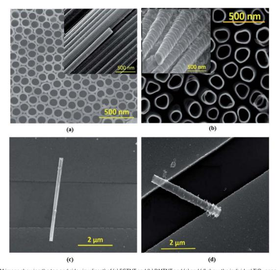
Fig. 1 FESEM image showing the top and side view (inset) of (a) EGTNT and (b) DMTNT and (c) and (d) show the individual  $TiO_2$  nanotube devices of EGTNT and DMTNT, respectively, on Au electrodes on top of the  $SiO_2/Si$  substrate.
