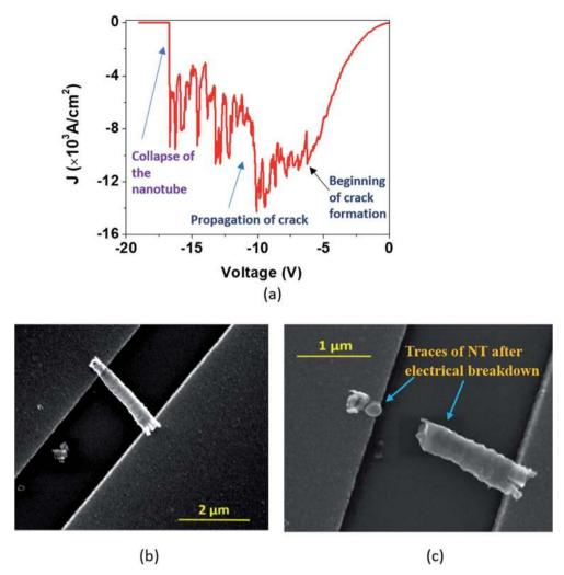
Fig. 6 (a) In the 'Model A' breakdown, the J-V curve displays features of an exponential rise in J along with nonlinearity before the verge of breakdown and reveals a stepwise fall of J during the electrical breakdown. SEM images exhibit a single DMTNT (b) before and (c) after the breakdown.
