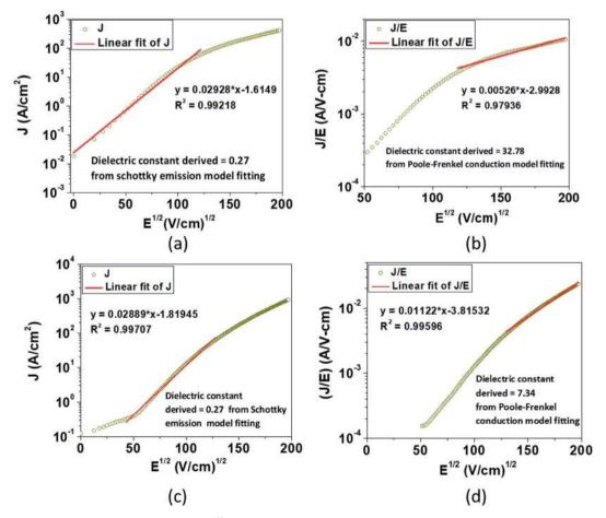
Fig. 3 The experimental semi-logarithm plot of J vs.  $E^{1/2}$  according to eqn (1) for (a) EGTNT and (c) DMTNT at 290 K in the lower bias region; the experimental semi-logarithm plot of (J/E) vs.  $E^{1/2}$  according to eqn (2) for (b) EGTNT and (d) DMTNT at 290 K in the higher electric field area. The red straight line denotes the fitting curve to those specified equations in a fixed range of the electric field.
