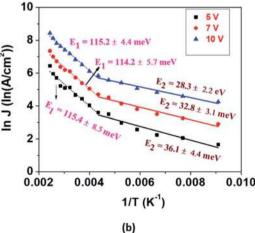
Fig. 4 Logarithm of current density (J) as a function of the reciprocal of the temperature between 110 K and 410 K at 3 different bias voltages (a) for individual EGTNT and (b) for individual DMTNT showing intermediate deep and shallow donor levels  $E_1$  and  $E_2$ , respectively. The symbols are the experimental data and the straight lines and dotted lines are the linearly fitted curves to the data.
