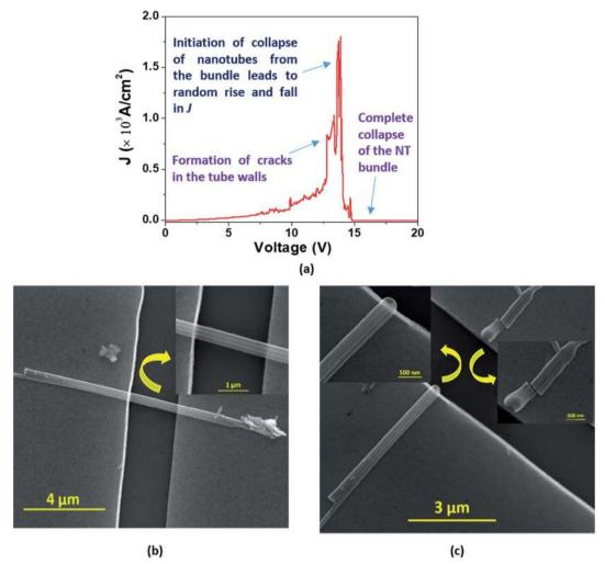
Fig. 9 (a) In the 'Model C' breakdown, the J-V curve displays mixed features of nonlinearity along with sudden big steps in J before the breakdown point which may be the characteristics for breaking of the bridge between the nanotubes in the bundle. SEM images exhibit a bundle of 3 EGTNT (b) before and (c) after the breakdown; magnified SEM images are also displayed in the insets.
