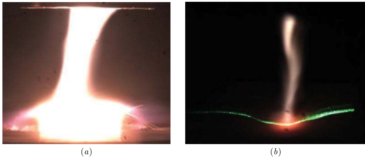
Figure 1. (a) Carbon sample with nitrogen plasma jet and sublimate puffs. (b) Sample shape during sublimation under argon plasma jet, the profile of the resulting cavity is visualized using a green laser knife.
