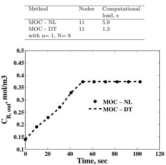
Fig. 3. Dynamic response of adiabatic FBR for 20% step down in inlet velocity using nonlinear integration method and DT method.
