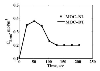
Fig. 4. Dynamic response of adiabatic FBR for 70% step down in inlet velocity using nonlinear integration method and DT method. Nu - number of terms in numerator, Dn - number of terms in denominator and n - number of sub-domains
