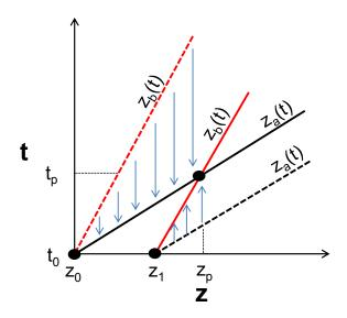
Fig. 1. Schematic figure showing characteristic lines starting from two different points in t-z plane
