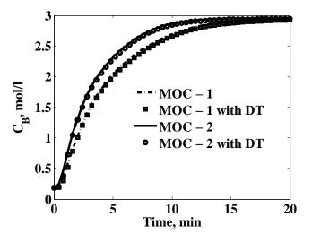
Fig. 5. Dynamic response of countercurrent PFR for 20% step up in inlet temperature of countercurrent heating fluid. DT is used with k = 0, 1, 2
