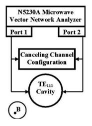
FIG. 1. Block diagram of the experimental arrangement for MFE technique.
