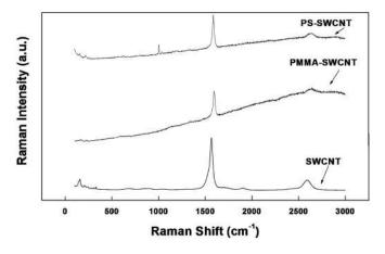
FIG. 2. Raman spectra for SWCNT, 0.5% w/w loaded SWCNT in PS and 0.5% w/w loaded SWCNT in PMMA.
