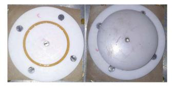
Figure 1. Teflon mould for a ring-shaped specimen.
