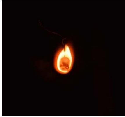
(c) volatiles-char oxidation around Oorja pellet at 270 \text{ s}^{-1} with 60% \text{O}_2 and 40% \text{CO}_2 .
