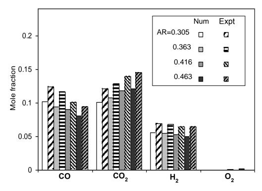
Figure 10. Comparison of predicted and measured product gas composition [12]
