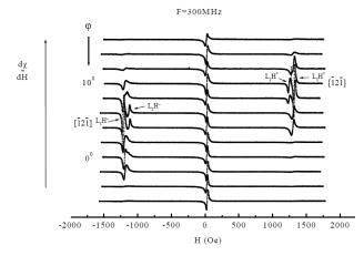
**Fig. 2.** Variation of the derivative of magnetic susceptibility with quasinormal external ( $\theta_H = 1$  degree) field for a range of azimuthal angles ( $\phi_H$ ) separated by an interval of 2 degrees. (F = 300 MHz and T= Ambient).
