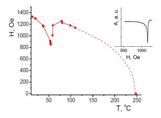
**Fig. 3.** Temperature dependence of the measured values of the transition field of the film to the saturation state.
