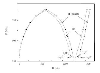
Fig.1. Experimental frequency-field dependence of FMR lines. The field is perpendicular to the surface of the film. (Dependence with a negative field is inverted to the positive axis).
