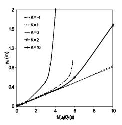
FIG. 4. The dependence of shock formation distance on the initial slope for various values of density gradient (*K*) for a linear density profile ( $\rho$ =1 +*Ky*). The value of  $B/\rho$  is kept constant as 1. Note that for the case of *K* =-1, shock forms only for high values of  $|u_1(0)|$ .
