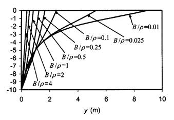
FIG. 1. Evolution of a compression wave front for various values of  $B/\rho$  for a linear density profile  $(\rho=1+y)$ ;  $|u_1(0)|=0.1$ .
