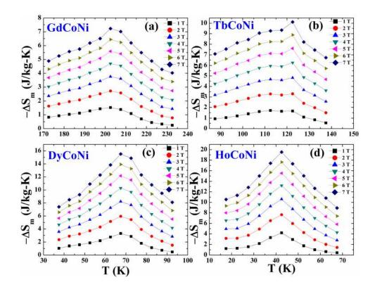
FIG. 2. Isothermal magnetic entropy change vs temperature of RCoNi (R = Gd, Tb, Dy, and Ho) compounds for various magnetic field changes.
