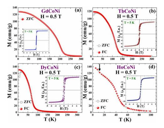
FIG. 1. Magnetization vs temperature of RCoNi (R = Gd, Tb, Dy, and Ho) compounds in applied field of 0.5 T [ZFC—zero-field cooled magnetization and FC—field cooled magnetization]. Inset shows magnetization vs field data.
