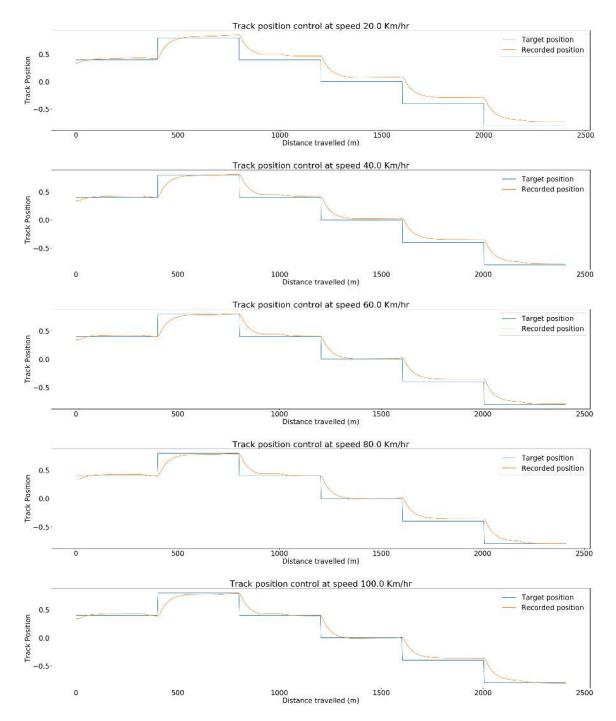
Figure 11: This plot demonstrates the position control accuracy and convergence over *distance* at different speeds of the PID controller used in our experiments. The track used is the "f-speedway" oval track and PID\_latency is set to 5. The plot covers the range of speeds used in our experiments.
