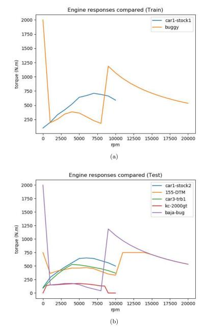
Figure 3: Variation of torque with engine RPM of cars studied in Experiment 2. (a) Torquevs-RPM of the cars that we present our agent to drive during training with equal probability. (b) Torque-vs-RPM of the cars that we test our agent on.
