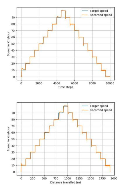
Figure 9: Speed control accuracy and convergence of our PID controller at different initial speeds over time-steps and distance travelled. The PID\_latency is set to 5. The track used in this study is the "f-speedway" oval track. The lane-position command is fixed at 0.0 which refers to the center of the track.
