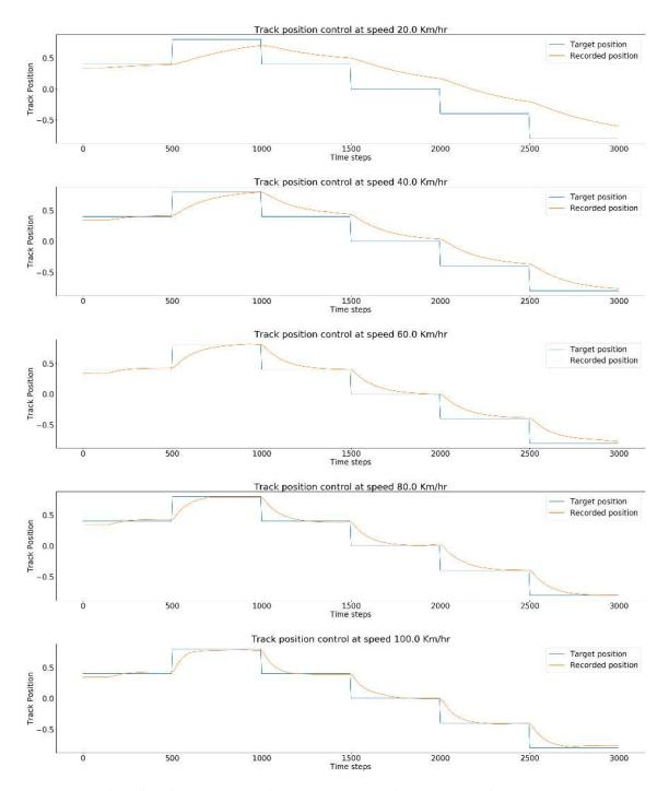
Figure 10: This plot demonstrates the position control accuracy and convergence over *time* at different speeds of the PID controller used in our experiments. The track used is the "f-speedway" oval track and PID\_latency is set to 5. The plot covers the range of speeds used in our experiments.
