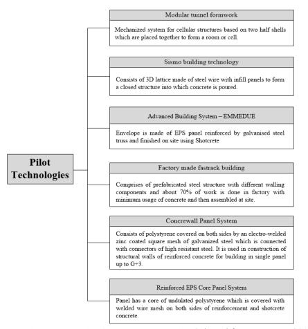
Figure 2: Pilot technologies for Low-cost Housing (adapted from BMTPC, 2015)
