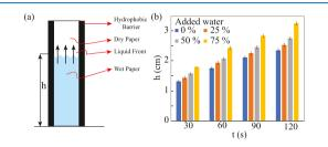
**Figure 4.** (a) Schematic of the paper strip for measuring the capillary height. (b) Change in the capillary height due to change in the water concentration at four different time intervals. Four different colors are showing the different concentrations of added water at a particular time. With the increase of the water concentration, the capillary height is also increased.
