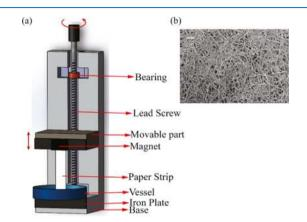
**Figure 6.** (a) Schematic of the experimental setup, which includes different parts such as bearing, lead screw, iron plate, magnets, etc. (b) SEM image of Whatman filter paper grade 4. Reprinted (adapted) with permission from ref 32. Copyright (2020) American Chemical Society.
