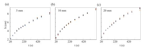
Figure 7. Graphical representation of capillary rise height and time for five repeated experiments in the case of (a) 5 mm, (b) 10 mm, and (c) 20 mm width paper strips.
