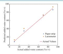
**Figure 5.** Comparison between the lactometer readings and paper strip readings (after 2 min). The actual values of the water content are shown by the red line.
