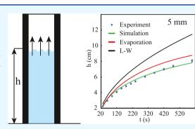
added water content in milk. We used milk as a liquid food and found the added water content from the change in the capillary height at different concentrations of milk. Finally, results obtained from the paper-based device were verified with the commercially available lactometer data.
