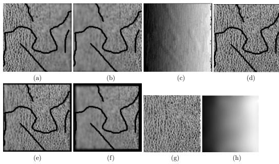
Fig. 1. (a,b) Frames 1 and 40 (unscaled stack). (c,d) Reconstructed depth profile and focused image using [1]. (e,f) Frames 20 and 40 from scaled stack. (g,h) Inpainted focused image and completed depth profile, respectively, using our method.
