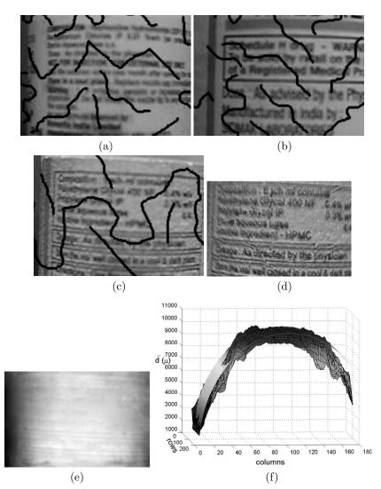
$\label{eq:Fig. 4. (a,b,c) Observations corresponding to the second frame for three different specimens. (d) Inpainted focused image corresponding to specimen (c). (e) Completed depth map. (f) Cylindrical fit to the estimated depth profile.$
