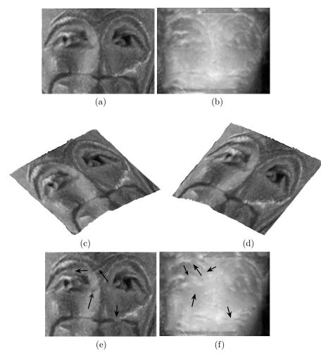
Fig. 5. (a) Inpainted focused image. (b) Inpainted depth map. (c,d) Novel view depiction. (e,f) Inpainted focused image and depth map, respectively, obtained using the observations in Figs. 2(c) and 2(d).
