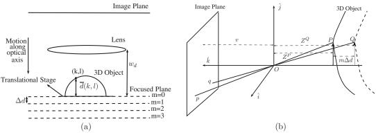
Fig. 3. (a) Working principle of SFF. (b) Schematic showing mechanism of structure-dependent pixel motion in SFF.
