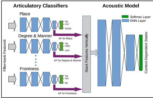
Figure 3: **DNN-joint-est**: Proposed technique of joint estimation of articulatory classifiers and acoustic model.
