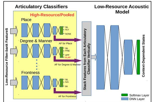
Figure 5: **Cross-DNN-joint-est**: Joint estimation framework for articulatory classifiers trained with high-resource/pooled data and acoustic model for low-resource language.
