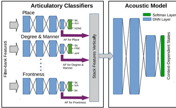
Figure 1: **DNN-sep**: Articulatory classifiers trained separately and are used to extract articulatory features for acoustic modeling.
