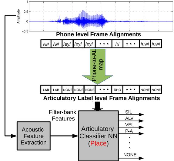
Figure 2: *Block schematic of training an articulatory classifier for place of articulation.*
