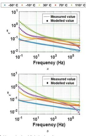
**Fig. 18** Measured and modelled  $\varepsilon''$  values of (a) Virgin and, (b) 8 kGy gamma irradiated specimens
