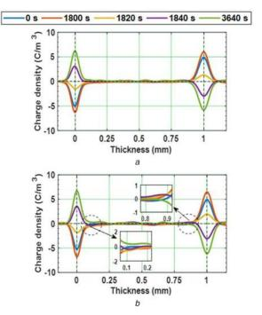
**Fig. 11** Space charge distribution under polarity reversal from positive to negative DC field stress in
