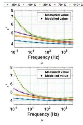
**Fig. 17** Measured and modelled  $\varepsilon'$  values of (a) Virgin and, (b) 8 kGy gamma irradiated specimens
