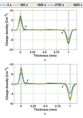
**Fig. 9** Space charge distribution during poling in (a) Virgin and, (b) 8 kGy irradiated specimens under 10 kV negative DC voltage
