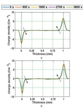
**Fig. 5** Space charge distribution during poling in (*a*) Virgin and, (*b*) 8 kGy gamma-irradiated epoxy micro-nanocomposites under 10 kV positive DC voltage
