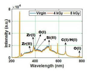
Fig. 21 Emission spectra of virgin and gamma irradiated epoxy nanomicro composites
