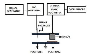
Fig. 1 Surface potential measurement setup
