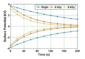
Fig. 14 Surface potential decay characteristics of virgin and gamma irradiated specimens under positive and negative DC corona charging
