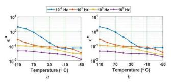
**Fig. 20** *Temperature variation in*  $\varepsilon''$  *values of* (a) Virgin and, (b) 8 kGy gamma irradiated specimens
