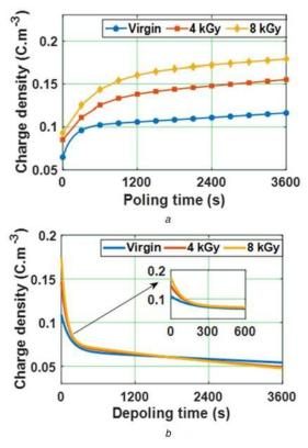
Fig. 8 Average space charge density of virgin and gamma-irradiated specimens during
