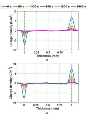
**Fig. 7** Space charge distribution during depoling of (a) Virgin and, (b) 8 kGy gamma-irradiated epoxy micro-nanocomposites after reduction of 10 kV positive DC voltage
