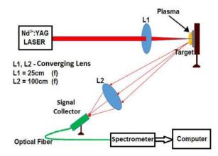
Fig. 2 Experimental setup of LIBS study
