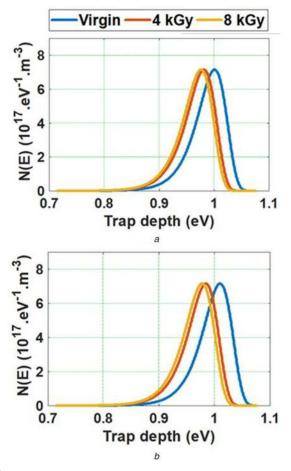
Fig. 15 Trap distribution characteristics of virgin and gamma irradiated specimens under
