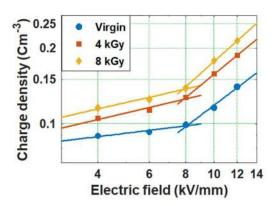
**Fig. 4** *Characteristic plot of average space charge density as a function of the applied electric field*
