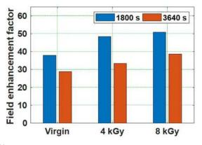
Fig. 13 Field enhancement factor of virgin and gamma-irradiated epoxy nanocomposites
