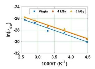
Fig. 19 Arrhenius plot of test specimens
