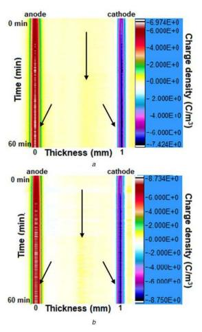
**Fig. 6** Space charge evolution during poling of (a) Virgin and, (b) 8 kGy gamma-irradiated epoxy micro-nanocomposites under 10 kV positive DC voltage
