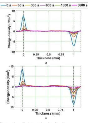
**Fig. 10** Space charge distribution during depoling of (a) Virgin and, (b) 8 kGy irradiated epoxy specimens after reduction of 10 kV negative DC voltage
