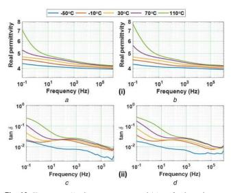
**Fig. 16** Variation in (i) relative permittivity and (ii) tan  $\delta$  values of (a) Virgin and, (b) 8 kGy gamma irradiated specimens
