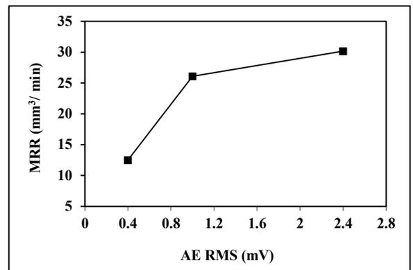
Fig. 7. (c) AE RMS vs. MRR
