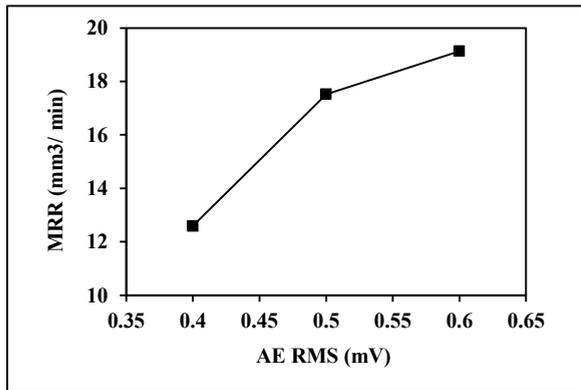
Fig. 6. (c) AE RMS vs. MRR
