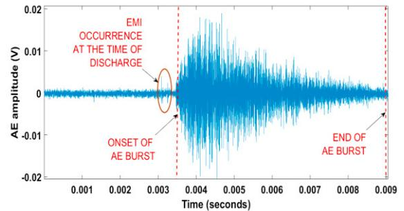
Fig 4. AE burst signal
