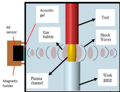
Fig. 2. Side view of the dielectric tank fitted with AE sensor
