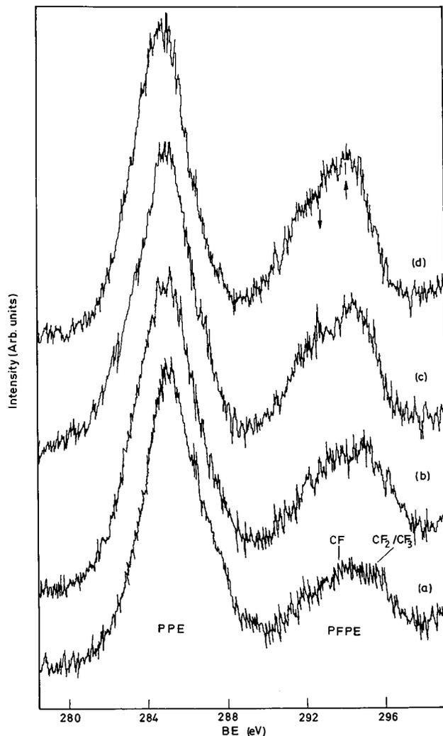
FIG. 1. X-ray photoelectron spectrum of the C 1s region of a mixture of perfluoropolyether and polyphenylether in the 1:100 volume ratio at various electron take-off angles. The various features are indicated. (a) 80, (b) 50, (c) 30, (d) 10°. Note the increase in intensity of the CF<sub>2</sub>/CF<sub>3</sub> feature as the take-off angle is decreased. Arrows show the direction of intensity variation.
