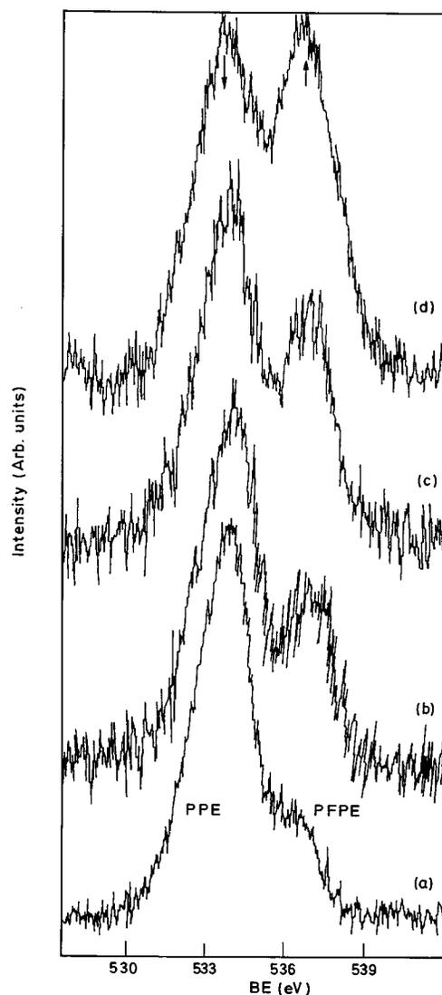
FIG. 2. X-ray photoelectron spectrum of the O 1s region of a mixture of perfluoropolyether and polyphenylether in the 1:100 volume ratio at various electron take-off angles. (a) 80, (b) 50, (c) 30, (d) 10°. Arrows indicate the direction of intensity variation.
