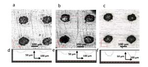
Fig. 9 Confocal microscopic images showing different dimple aspect ratio of (a) 0.1, (b) 0.2 and (c) 0.3 ( $D = 130 \mu$ m,  $A_d = 16\%$  for all the samples).
