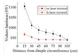
Fig. 14 Measurement of Vickers hardness as a function of distance from the dimple circumference for nanosecond and femtosecond pulsed laser textured ring sample ( $D = 130 \mu m$ ,  $A_d = 16\%$  and a = 0.2 for both the samples).
