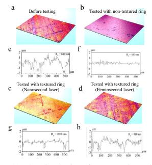
Fig. 15 Three-dimensional surface topography and corresponding roughness of liner surface at its dead centre (a) Before testing, (b) After testing with non-textured sample, (c) After testing with nanosecond pulsed laser textured sample ( $D = 130 \ \mu\text{m}$ ,  $A_d = 16\%$  and a = 0.2) and (d) After testing with femtosecond pulsed laser textured sample ( $D = 130 \ \mu\text{m}$ ,  $A_d = 16\%$  and a = 0.2).
