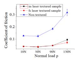
Fig. 13 Coefficient of friction graph for non-textured, nanosecond pulsed laser textured ( $D = 130 \ \mu m$ ,  $A_d = 16\%$  and a = 0.2) and femtosecond pulsed laser textured ( $D = 130 \ \mu m$ ,  $A_d = 16\%$  and a = 0.2) ring samples.
