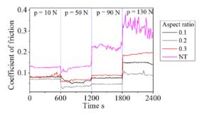
Fig. 10 Typical coefficient of friction graph obtained from the tribology test showing the influence of different dimple aspect ratio for the stepwise increase of load ( $D = 130 \ \mu m$  and  $A_d = 16\%$  for all the samples).
