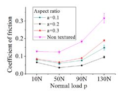
Fig. 11 Average coefficient of friction as a function of load for the non-textured and textured samples of different dimple aspect ratios 0.1, 0.2 and 0.3. ( $D = 130 \,\mu\text{m}$  and  $A_d = 16\%$  for all the samples).
