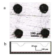
Fig. 12 (a) Femtosecond laser textured sample and (b) corresponding dimple profile ( $D = 130 \ \mu m$ ,  $A_d = 16\%$  and a = 0.2).
