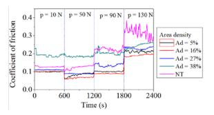
Fig. 6 Typical coefficient of friction graph as a function of time for non-textured and textured samples of different dimple area density for the stepwise increase of load ( $D = 130 \ \mu m$  and a = 0.3 for all the samples). NT: Non-textured sample.
