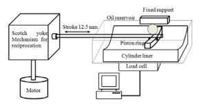
Fig. 2 Reciprocating type friction testing tribometer.
