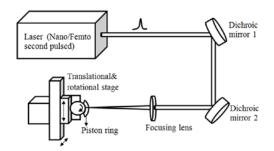
Fig. 1. Laser texturing set up.
