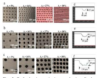
Fig. 5 Confocal microscopic images showing dimple diameter of (a)  $D = 40 \ \mu\text{m}$ , (b)  $D = 80 \ \mu\text{m}$ , (c)  $D = 130 \ \mu\text{m}$  and the corresponding profile of the samples with dimple depth of (d)  $d_d = 12 \ \mu\text{m}$ , (e)  $d_d = 25 \ \mu\text{m}$ , (f)  $d_d = 40 \ \mu\text{m}$ . All samples were maintained at an aspect ratio a = 0.3. Ad: Dimple area density varying from 5% to 38%.
