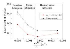
Fig. 8 Schematic of Stribeck curve for various lubricating regimes ( $D = 130 \ \mu m$  and  $p = 50 \ N$ ).
