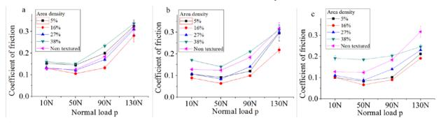
Fig. 7 Average coefficient of friction as a function of normal load corresponding to different values of area density for the dimple diameter of (a) 40  $\mu$ m, (b) 80  $\mu$ m and (c) 130  $\mu$ m.
