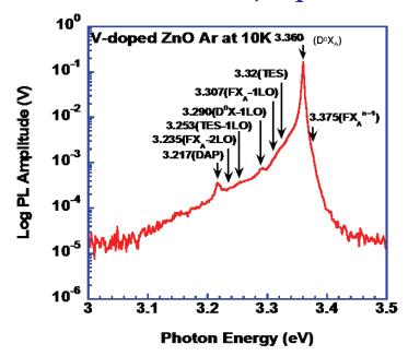
**Figure 7.** Logarithmic plot of the low-temperature PL spectrum of V:ZnO films grown in Ar atmosphere at 10 K.
