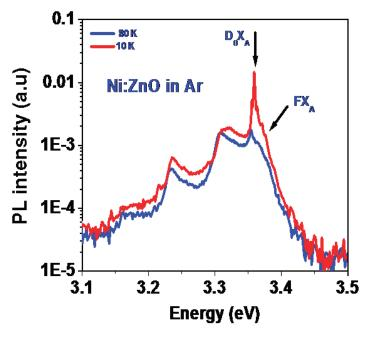
**Figure 9**. Temperature dependence of excitonic emission in the PL spectra of Ni:ZnO.
