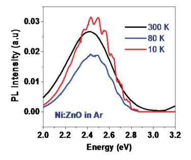
**Figure 6.** Temperature dependence of visible spectra of Ni:ZnO films grown in Ar atmosphere.
