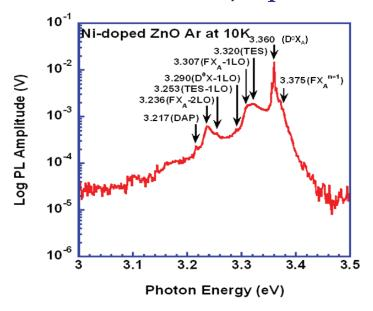
**Figure 8.** Logarithmic plot of the low-temperature PL spectrum of Ni:ZnO grown in Ar atmosphere at 10 K.
