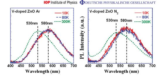
Figure 5. Temperature dependence of visible emission from V-doped samples.
