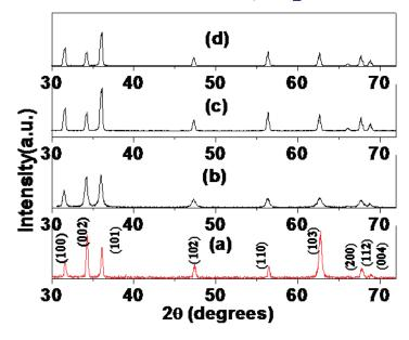
**Figure 1.** XRD patterns of as-grown Ni-doped ZnO film in (a) Ar, (b)  $N_2$  and V-doped ZnO film in (c) Ar, (d)  $N_2$ .
