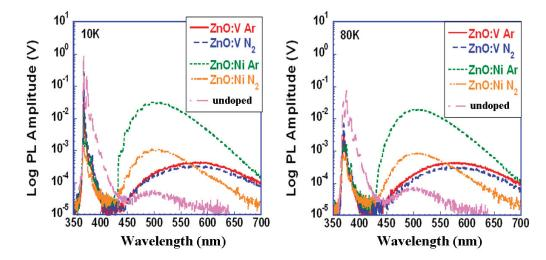
**Figure 4.** Low-temperature PL spectra of Ni:ZnO and V:ZnO thin films grown in Ar and  $N_2$  atmospheres.
