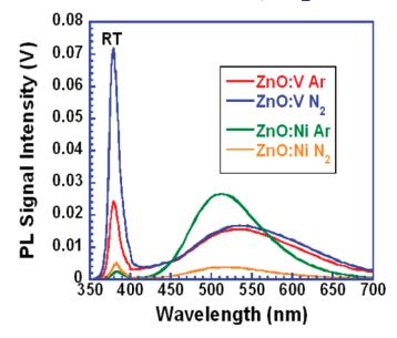
**Figure 3.** Room temperature PL spectra of Ni:ZnO and V:ZnO thin films grown in Ar and  $N_2$  atmospheres.
