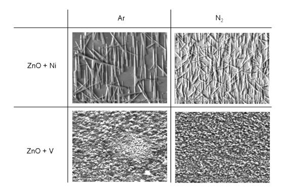
Figure 2. SEM images of Ni- and V-doped films grown in Ar and N<sub>2</sub>.
