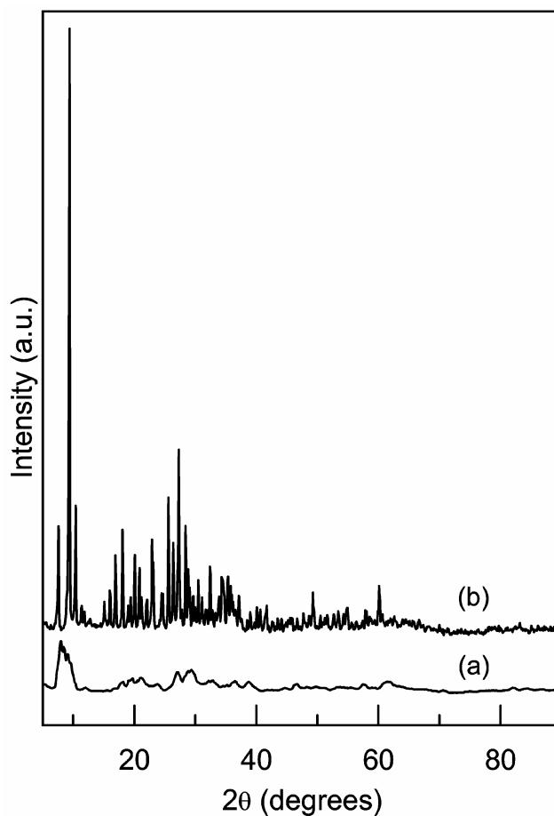
**Figure 2.** Powder XRD pattern of (a)  $\text{H}_3\text{PW}_{12}\text{O}_{40}n\text{H}_2\text{O}$ , and (b)  $[\text{BmIm}]_3[\text{PW}_{12}\text{O}_{40}]$  hybrid molecular material.
