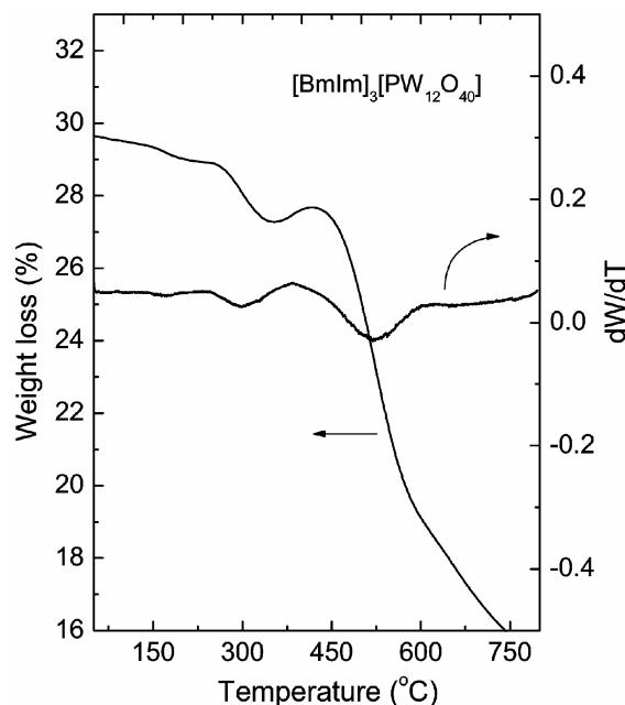
**Figure 5.** TGA of  $[\text{BmIm}]_3[\text{PW}_{12}\text{O}_{40}]$  hybrid molecular material.
