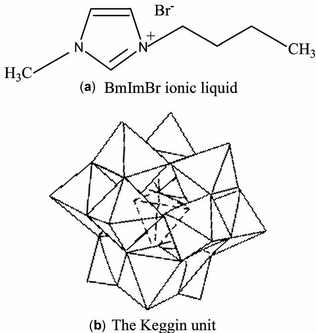
**Figure 1.** (a) 1-Butyl 3-methyl imidazolium bromide (BmImBr), and (b) PW<sub>12</sub>O<sub>40</sub><sup>3−</sup> Keggin molecular anion.
