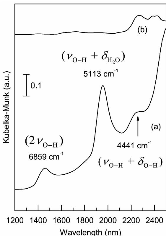
**Figure 8.** Near IR spectra of (a) H<sub>3</sub>PW<sub>12</sub>O<sub>40</sub>·nH<sub>2</sub>O, and (b) [BmIm]<sub>3</sub>[PW<sub>12</sub>O<sub>40</sub>] hybrid molecular material.
