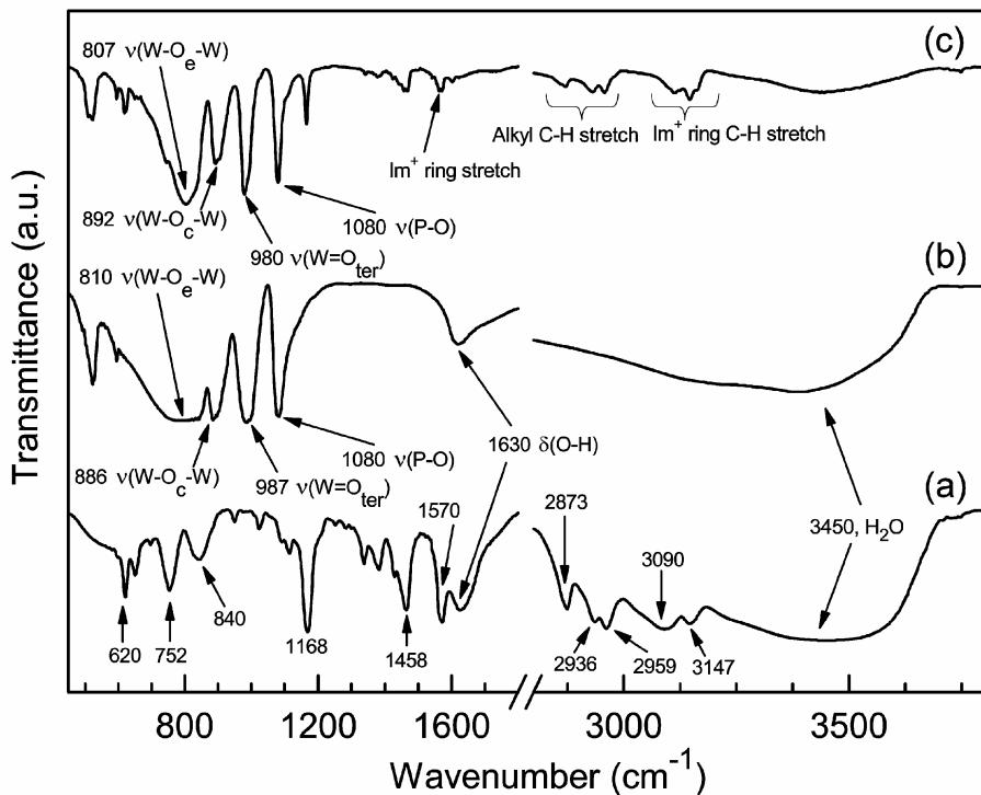
**Figure 3.** FTIR spectra of (a) 1-butyl 3-methyl imidazolium bromide ( $\text{BmImBr}$ ) ionic liquid, (b)  $\text{H}_3\text{PW}_{12}\text{O}_{40}n\text{H}_2\text{O}$ , and (c)  $[\text{BmIm}]_3[\text{PW}_{12}\text{O}_{40}]$  hybrid molecular material.
