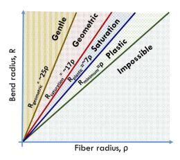
Fig. S7: Parametric space of bend radius and fiber radius showing the different regimes of bending. The solid lines represent constant ratios of bend radius to fiber radius.
