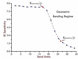
Fig. 4: RI sensitivity of U-bent POF for various bend ratios, considering  $n_{\rm med}$  =1.37. (RI Sensitivity is estimated as change in normalized refractive loss (dB) for a change in the RI of medium with respect to water as reference.)
