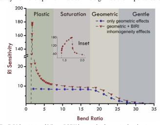
Fig. 7: RI Sensitivity of 0.5 mm POF U-bent probe, for varying bend ratios. Inset: RI Sensitivity for bend ratios between  $1.4\,\mathrm{and}~2.1$
