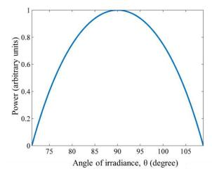
Fig. S1: Power distribution for rays coupled to an optical fiber using a microscopic objective
