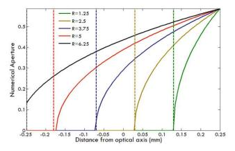
Fig. 2: Simulation results obtained for a plastic optical fiber of 0.5 mm fiber core diameter. The NA across the various bend radii for  $n_{med}$  of 1.37 was calculated using analytical equation and compared with the width of propagation estimated using ray optics model
