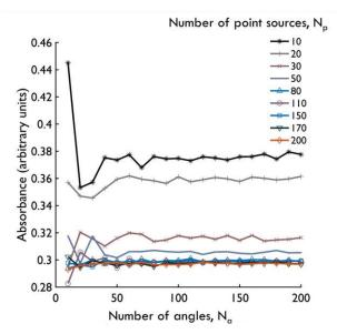
Fig. S2: Absorbance simulated using the 2D ray tracing model for a 500  $\mu m$  POF U-bent probe with a bend diameter of 3.0 mm and aqueous medium RI of 1.36. Simulations have been carried out for varying number of ray positions and angles of propagation to verify convergence of resultant absorbance
