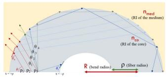
Fig. 1: Ray optics model for evaluation of refractive losses in a U-bent fiber optic sensor
