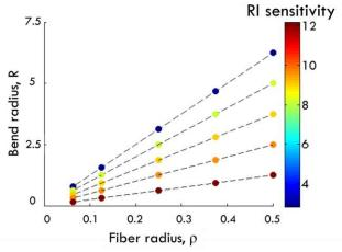
Fig. S6: 2D scatter plot with RI sensitivity values in color, obtained for a plastic optical fiber of bend radii and fiber radii in the range of (0.3125 - 12.5) and (0.125 to 1.00 mm) respectively. The dashed lines represent constant bend ratios (ratio of bend radius to fiber radius).
