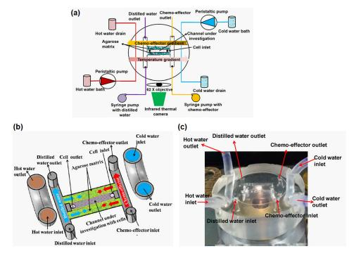
FIG. 1. (a) Sketch of the experimental setup for the cell migration study under imposed competing chemical and thermal gradients. (b) Schematic illustration of the channels in the device. (c) Schematic view of the microfluidic device under working conditions.
