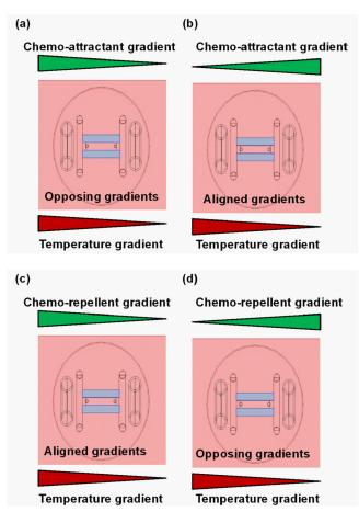
FIG. 2. Combined gradient generation within the microfluidic device. (a) Opposing gradients of the attractant (sorbitol) and temperature. (b) Aligned gradients of the attractant and temperature (c) Aligned gradients of the inhibitor ( $NiSO_4$ ) and temperature. (d) Opposing gradients of the inhibitor and temperature.
