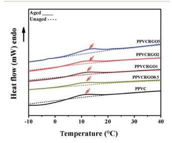
Fig. 8 Physical aging of PPVC/RGO nanocomposites at  $T_a = -10~^{\circ}\text{C}$  during 15 h.
