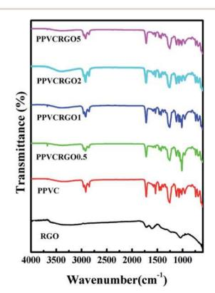
FTIR spectra of RGO and PPVC/RGO nanocomposites.
