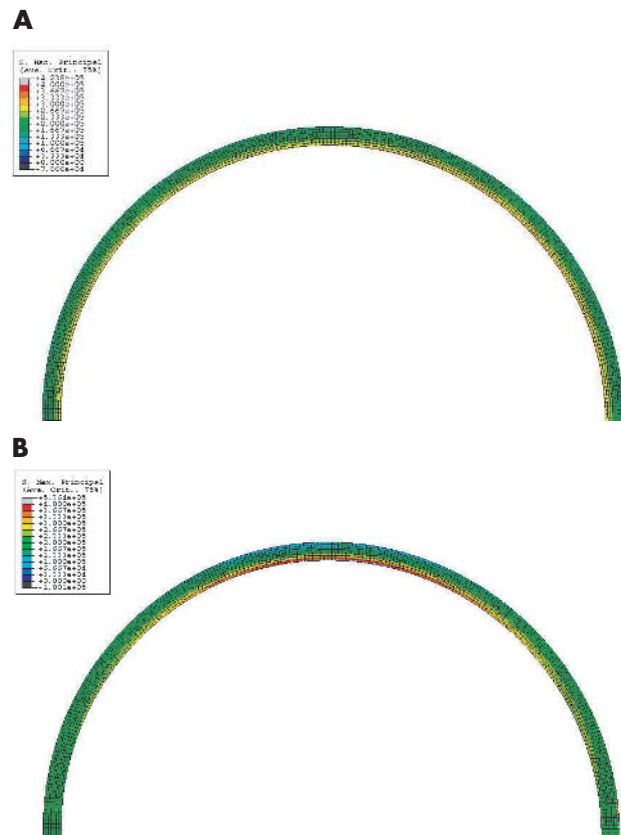
Figure 3 (A) Stress distribution in a circular lumen. Note the uniform stress distribution of the lumen. Only the top half of the figure is shown. (B) Stress distribution in an elliptical lumen. Note the higher stresses towards the major axis. Red is the highest and blue is the lowest.
