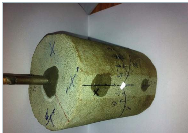
FIGURE 17. Fracture orientation as seen on sample surface.
