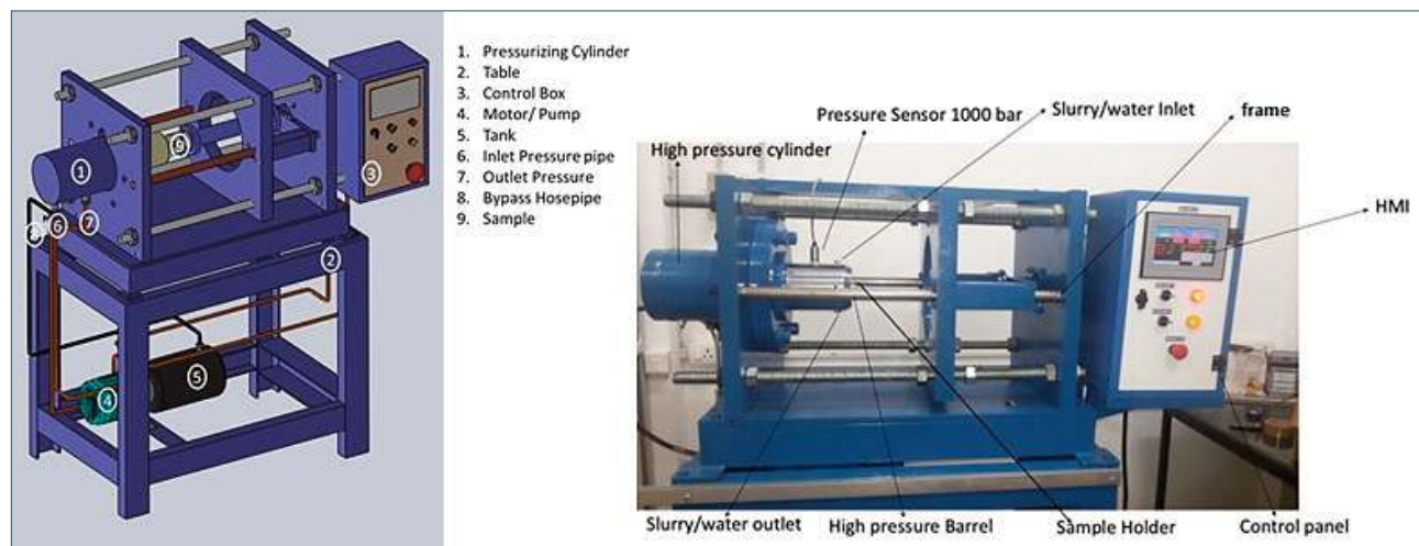
FIGURE 4. Laboratory Scale Hydraulic fracturing setup.
