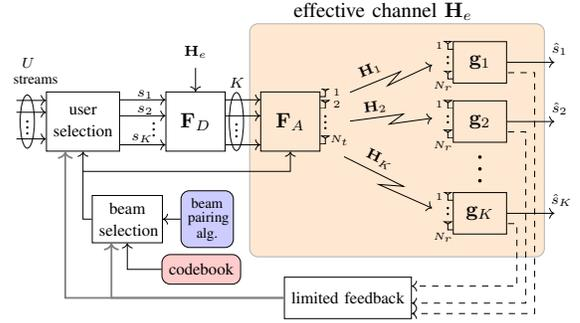
Fig. 1: Downlink limited feedback hybrid beamforming system
