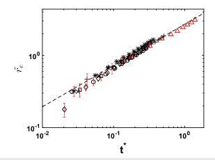
**FIG. 8**. Variation of the dimensionless excess outer radius of the rim  $\tilde{r}_e = r_e(t)/R$  with the dimensionless time  $t^* = t/t_c$ . For water: +, R = 0.175 mm; \*, R = 0.47 mm;  $\bigcirc$ , R = 2.32 mm; and  $\square$ , R = 1.47 mm. For other fluids:  $\diamondsuit$ , R = 0.7 mm, GW55; ×, R = 1.16 mm, ethanol;  $\triangle$ ,  $R = 25 \ \mu$ m, ethanol from San Lee *et al.*;<sup>17</sup> and --,  $\tilde{r}_e = 2.7t^{*4/7}$  (31).
