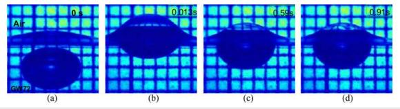
FIG. 4. The interaction of a rising bubble of R = 2.2 mm (Bo = 0.9) with the free surface in GW72. (a) Approach to the free surface, [(b) and (c)] oscillation at the free surface, and (d) the static configuration. For similar Bo, the bubble collapses 4 s after (d). Grid size is 1 mm.
