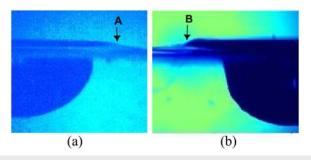
**FIG. 11.** Comparison of the swell in a high viscosity fluid with that in water at approximately 1.4 ms after the thin film rupture. (a) A smooth swell for R = 2.4 mm (Oh = 0.27,  $R/R_{\mu\sigma} = 13.7$ ) in GW86.8. Image width is 5.1 mm. (b) A sharp swell for R = 2.32 mm (Oh = 0.0025,  $R/R_{\mu\sigma} = 16 \times 10^4$ ) in water. Image width is 4.63 mm.
