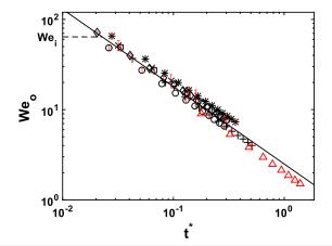
**FIG. 9.** Variation of the Weber number of expansion of the outer radius of the hole  $We_o$  with the dimensionless time  $t^* = t/t_c$ . For water: +, R = 0.175 mm; \*, R = 0.47 mm;  $\bigcirc$ , R = 2.32 mm; and  $\square$ , R = 1.47 mm. For other fluids:  $\diamondsuit$ , R = 0.7 mm, GW55; ×, R = 1.16 mm, ethanol;  $\triangle$ ,  $R = 25 \ \mu$ m, ethanol from San Lee *et al.*;<sup>17</sup> —,  $We_o = 2.5t^{*-6/7}$  (34); and --,  $We_i = 64$  (38).
