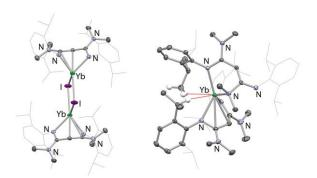
**Figure 11.** Molecular structures of  $\{[1^{Dipp}]Yb(\mu-I)\}_2$  and  $[1^{Dipp}]_2Yb$  in the solid state as determined by X-ray crystallography. Displacement ellipsoids drawn at 50 % probability level; most hydrogen atoms omitted and N-substituents drawn in wireframe format for clarity. The structure of  $\{[1^{Dipp}]Yb(\mu-I)\}_2$  is centrosymmetric; only one of the two independent components in the asymmetric unit is shown.
