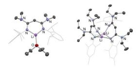
**Figure 5.** (left to right) Molecular structures of [1<sup>Dipp</sup>]Li(OEt<sub>2</sub>), and one of the molecules in the asymmetric unit of {[4<sup>Mes</sup>]Li]<sub>2</sub>, in the solid state as determined by X–ray crystallography. Displacement ellipsoids drawn at 50 % probability level; most H-atoms, minor disorder components and solvate molecules omitted and N-substituents drawn in wireframe format for clarity. Key metrical parameters are given in Table 3.
