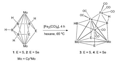
Scheme 1 Synthesis of dimolybdaborane cubane-type clusters 3 and 4.
