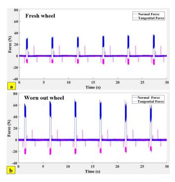
Fig. 4. Grinding Forces: (a) Fresh wheel; (b) Worn-out wheel
