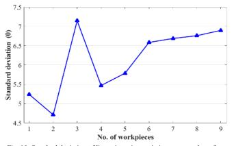
Fig. 10. Standard deviation of line orientation variation over number of ground workpiece
