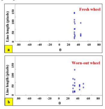
Fig. 8. Detection of line length and orientation: (a) Fresh wheel; (b) Worn-out wheel
