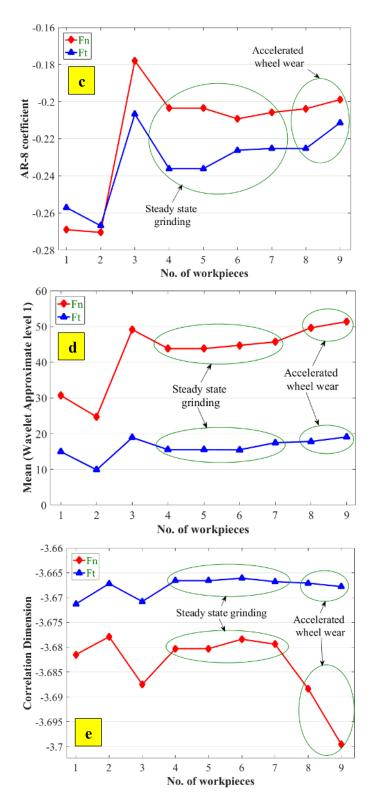
Fig. 5. Effective grinding force features: (a) Energy; (b) Mean; (c) AR-8 coefficient; (d) Mean wavelet level 1 approximate coefficient; (e) Correlation dimension
