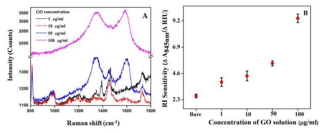
**Fig. 3.** (A) Raman scattering spectrum of BPOFs coated using different concentrations of GO solutions  $(1 \ \mu g/ml, 10 \ \mu g/ml, 50 \ \mu g/ml)$  and  $100 \ \mu g/ml)$  and incubation of 24 h followed by post heat treatment at 50 °C for 10 min. (B) RI sensitivity ( $\Delta A_{845nm}/\Delta RIU$ ) of BPOF probes without and with GO coating using varying concentration of aqueous GO solution.
