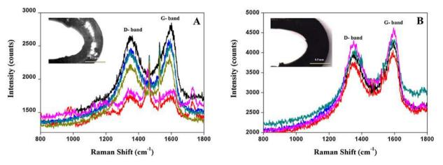
Fig. 2. Raman scattering spectra obtained from (A) bare and (B) HMDA functionalized BPOF probes coated with GO. The BPOF probes were heat treated after GO coating to improve GO adhesion. Raman scattering spectra were recorded at different points over a given sensor surface.
