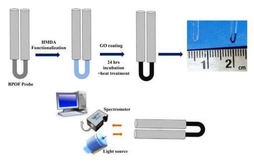
Fig 1. Schematic representation of the optical setup and photographic image of bare BPOF (left) and GO-BPOF probe (right).
