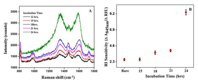
**Fig. 4.** (A) Raman scattering spectrum of BPOFs coated with GO solutions of concentration 100  $\mu$ g/ml at varying incubation time Includes 2, 4, 6, 12, 15, 18, 21 and 24 h followed by post heat treatment at 50 °C for 10 min. (B) RI sensitivity ( $\Delta A_{845nm}/\Delta RIU$ ) of bare and GO-BPOF probes using varying incubation time.
