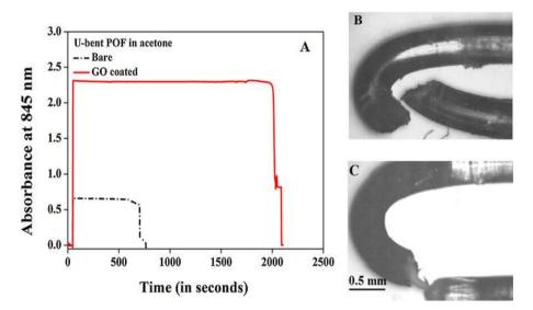
**Fig. 6.** Real time monitoring of optical absorbance response from bare and GO-BPOF probes dipped in acetone (at t = ~50 s). An abrupt drop in light intensity through the BPOF probes was observed indicating sudden fiber probe breakage. (B), (C) Microscopic image bare and GO-BPOF probes after dipping in acetone respectively.
