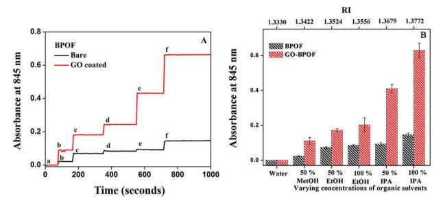
Fig. 5. (A) Temporal response and (B) Absorbance response at 845 nm wavelength obtained from bare and GO-BPOF subjected to organic solvents of varying concentrations including (a) Reference water, (b) 50% v/v MeOH, (c) 50% v/v EtOH, (d) 100% v/v EtOH, (e) 50% v/v IPA and (f) 100% v/v IPA.
