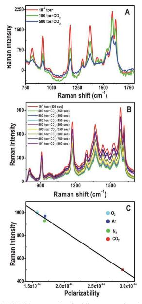
Fig. 3 (A) SERS spectrum collected at different concentrations of  $CO_2$ . (B) Change in SERS intensity of Au@MSA SL crystals under 500 Torr of  $CO_2$  at different time intervals. (C) Change in Raman intensity vs. polarizability of gases at 500 Torr  $(O_2, Ar, N_2 \text{ and } CO_2)$ .
