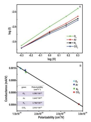
Fig. 2 (A) Plot of log current (mA) vs. log voltage (V) of the SL crystals upon exposure to gases, O2, Ar, N2, and CO2 at 500 torr. (B) Conductance (slope of I vs. V, in mA  $V^{-1}$ ) vs. polarizability (cm<sup>2</sup>  $V^{-1}$ ) of the corresponding gases. Table in the inset shows the polarizability of all the four gases under consideration.
