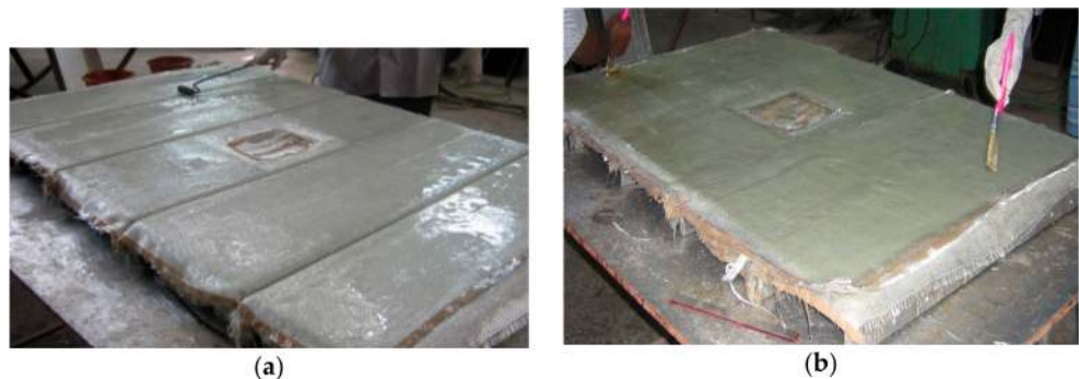
Figure 4. Casting of GFRP-stiffened composite plates. (a) Laying of the first three layers (b) Laying of last three layers.
