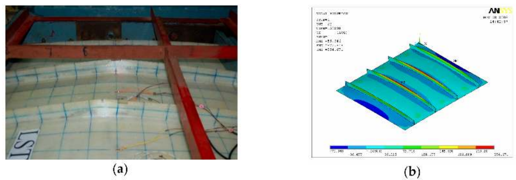
Figure 15. Failure of LSTP4. (a) Experiment (b) FEA.
