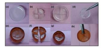
Fig. 7 a-d) Demonstration of self-healing property in 5 wt% Mesitylene gel disc from 1.4(S); e-h) similar images from its 5 wt% Tetralin gel.
