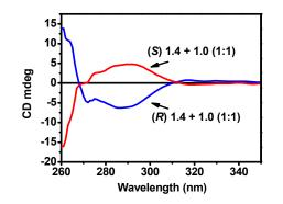
**Fig. 10** CD spectra showing chiral preferences of achiral dipeptide **1.0** in the gel state when used in combination with the chiral dipeptide **1.4** in R or S forms
