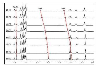
**Fig. 5** Variable temperature <sup>1</sup>H NMR spectra of **1.4** in Toluene-d<sub>8</sub> (5 wt%) showing evidences of hydrogen bonding involving NH and triazolyl protons during gelation.
