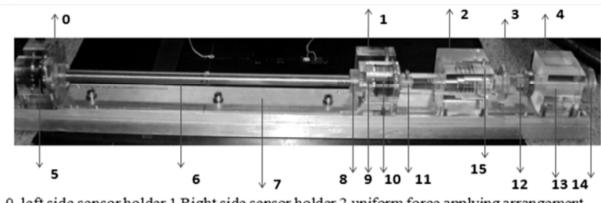
0. left side sensor holder, 1.Right side sensor holder, 2.uniform force applying arrangement,
