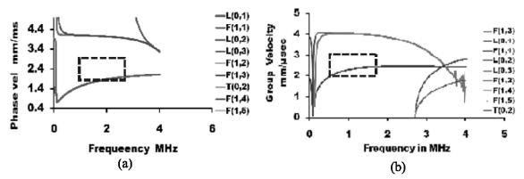
Fig. 2 : Dispersion curves for Zircalloy-4 tube (diameter 15.25mm and thickness 0.5 mm) (a) phase velocity, and (b) group velocity plots.
