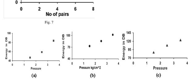
Fig. 8 : Pressure vs. reflected energy from welded tube based on table 2. (a). 90Ws, (b).110Ws, (c).150Ws
