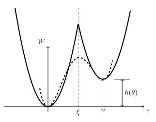
Figure 3: Energy per atom of the lattice as a function of the shear of the lattice  $\varepsilon$ . The free energy presented in Eq. (8) is shown as a function of the parameter  $\varepsilon$  as a dashed line. The solid lines represent a piecewise parabolic approximation.
