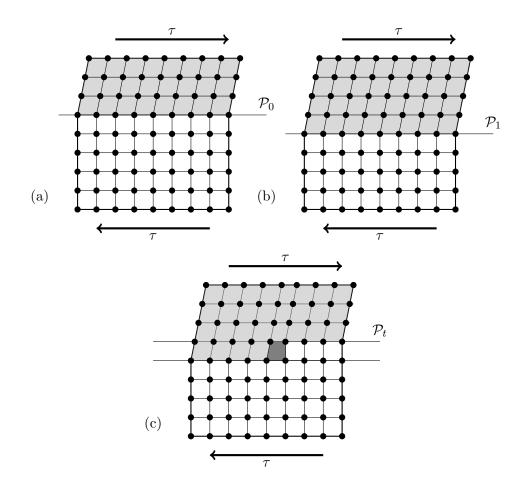
Figure 2: (a) The lattice showing the location of the phase boundary  $\mathcal{P}_0$ . (b) Phase boundary  $\mathcal{P}_1$  after motion by one lattice spacing. (c) Schematic of a ledge on the phase boundary. The ledge is shaded dark gray. The propagation of the ledge to the right results in a downward propagation of the phase boundary.
