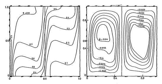
Figure 3 Isotherms and streamlines for XH=0.5;  $Ra_{\rm H}=10^6$ ; Pr=1
