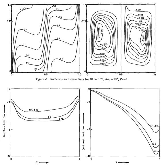
Figure 5 Variation of heat flux along the partition height Figure 6 Variation of heat flux along cold wall with XH with XH
