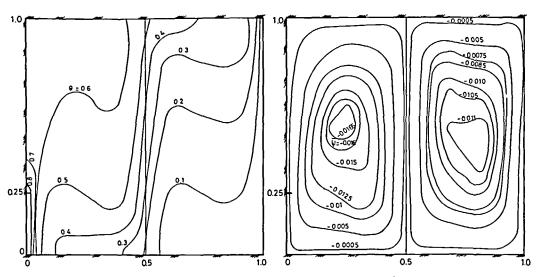
Figure 2 Isotherms and streamlines for XH=0.25;  $Ra_{\rm H}=10^6$ , Pr=1
