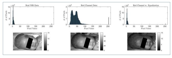
Fig. 3 Left: Real NIR data. Center: Red channel of RGB image. Right: Virtual NIR image. The top row shows histograms; the bottom row excerpts of the corresponding images. Note the different scale of the colorbar in the center image
