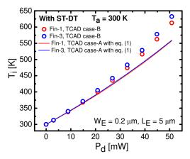
Fig. 2. Dissipated power-dependent true temperature  $(T_i)$  of  $1^{st}$  and  $3^{rd}$  finger in a five finger transistor. Circles correspond to case-B TCAD simulation. Solid lines are the results obtained following (1) from case-A TCAD simulations by exciting one finger at a time.
