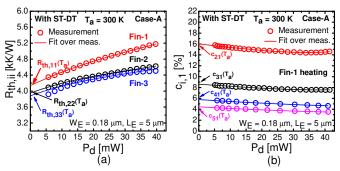
Fig. 5. Measured dissipated power-dependent (a) self-heating thermal resistance of  $1^{st}$ ,  $2^{nd}$  and  $3^{rd}$  finger, and (b) coupling coefficients obtained when only  $1^{st}$  finger is heating. Extracted  $R_{th,ii}(T_a)$  and  $c_{ij}(T_a)$  are also marked.
