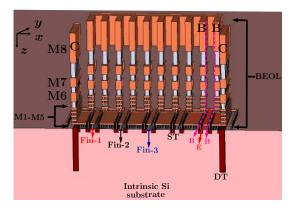
Fig. 1. 3D cross-sectional view of a five-finger TCAD structure of STMicroelectronics B55 process [12] containing shallow and deep trenches along with the eight metal layers (M1 to M8) in BEOL. A set of emitter (E), base (B), and collector (C) contacts are indicated for the rightmost corner finger.
