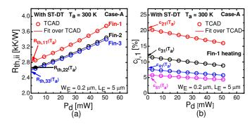
Fig. 3. Self-heating and thermal coupling results obtained from case-A TCAD simulations: (a)  $P_{d,i}$ -dependent self-heating thermal resistance  $R_{th,ii}$  of all three individually heating fingers (Fin-1, 2 and 3) and (b) coupling coefficients obtained for case-A when only  $1^{st}$  finger is heating (j=1) and rest are sensing. Ambient variables  $R_{th,ii}(T_a)$  and  $c_{ij}(T_a)$  are also indicated.
