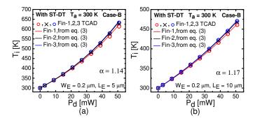
Fig. 4. A comparison of dissipated power-dependent temperatures  $T_i$ , at fingers 1, 2 and 3 obtained from the proposed extraction scheme (solid lines) against case-B TCAD simulation (symbols) for devices with emitter area  $(A_E)$  of (a)  $A_E=0.2\times 5~\mu m^2$  and (b)  $A_E=0.2\times 10~\mu m^2$ .
