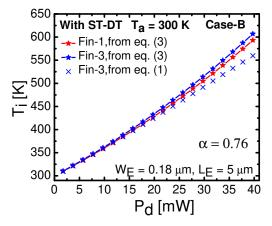
Fig. 6. Extracted values of true finger temperatures (star-lines) for  $1^{st}$  and  $3^{rd}$  finger of a five finger device from B5T technology [17]. An underestimated finger-3 temperature (crosses) obtained from a direct superposition of measured self-heating and thermal coupling temperatures is also shown for comparison.
