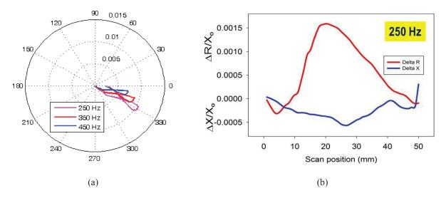
FIGURE 3. (a) Coil impedance plane trajectory for a sub-surface notch located 9 mm deep in 10 mm thick aluminium plate. (b) Change in normalized coil impedance at 250 Hz. Defect depth is 1 mm.
