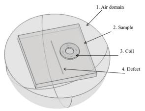
FIGURE 4. Schematic of the FEM model
