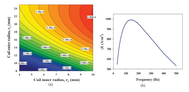
FIGURE 5. (a) Magnitude of magnetic field density, |B| at 150 Hz on the defect surface (S<sub>2</sub>) for varying coil inner ( $r_1$ ) and outer ( $r_2$ ) radii, ( $r_1$ : 4 mm to 10 mm;  $r_2$ : 8 mm to 25 mm); (b) induced current density at plate bottom for  $r_1 = 10$  mm,  $r_2 = 23$  mm, h=3 mm, d=0.5 mm.
