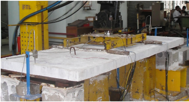
Fig. 5 Picture of a panel in test setup.
