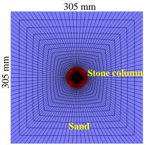
Fig. 4. Plan view of ordinary stone column installed at the center of shear box.
