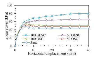
Fig. 6. Shear stress vs. displacement ( $\sigma_n = 75$  kPa).
