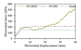
Fig. 7. Horizontal stress ( $\sigma_x$ ) developed above the shear plane.
