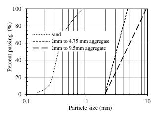
Fig.2. Grain size distribution of sand and aggregates.
