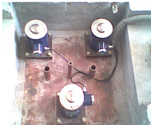
Fig. 1b. Drop mass setup – load cell arrangement.
