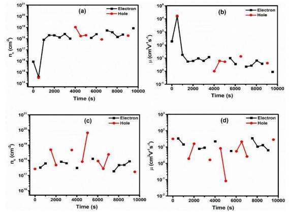
**Figure A3.** Photo Hall effect measurements (using HMS 7406) performed on 1 cm  $\times$  1 cm ITO/TiO<sub>2</sub> photocatalyst coated on quartz tube. Sheet carrier density (n<sub>s</sub>) and mobility ( $\mu$ ) at a function of time (t) when UV 254 nm is (a) and (b) on and (c) and (d) off.
